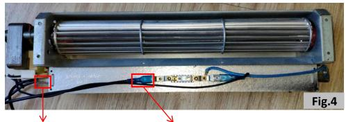
Here are two sets of heating. If one wire disconnects, one set will does not heat.
