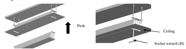
5. Install plastic cover panel (N) to complete the installation.
