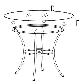
Place the table on the floor to check if it is stable before tightening bolts (E).
