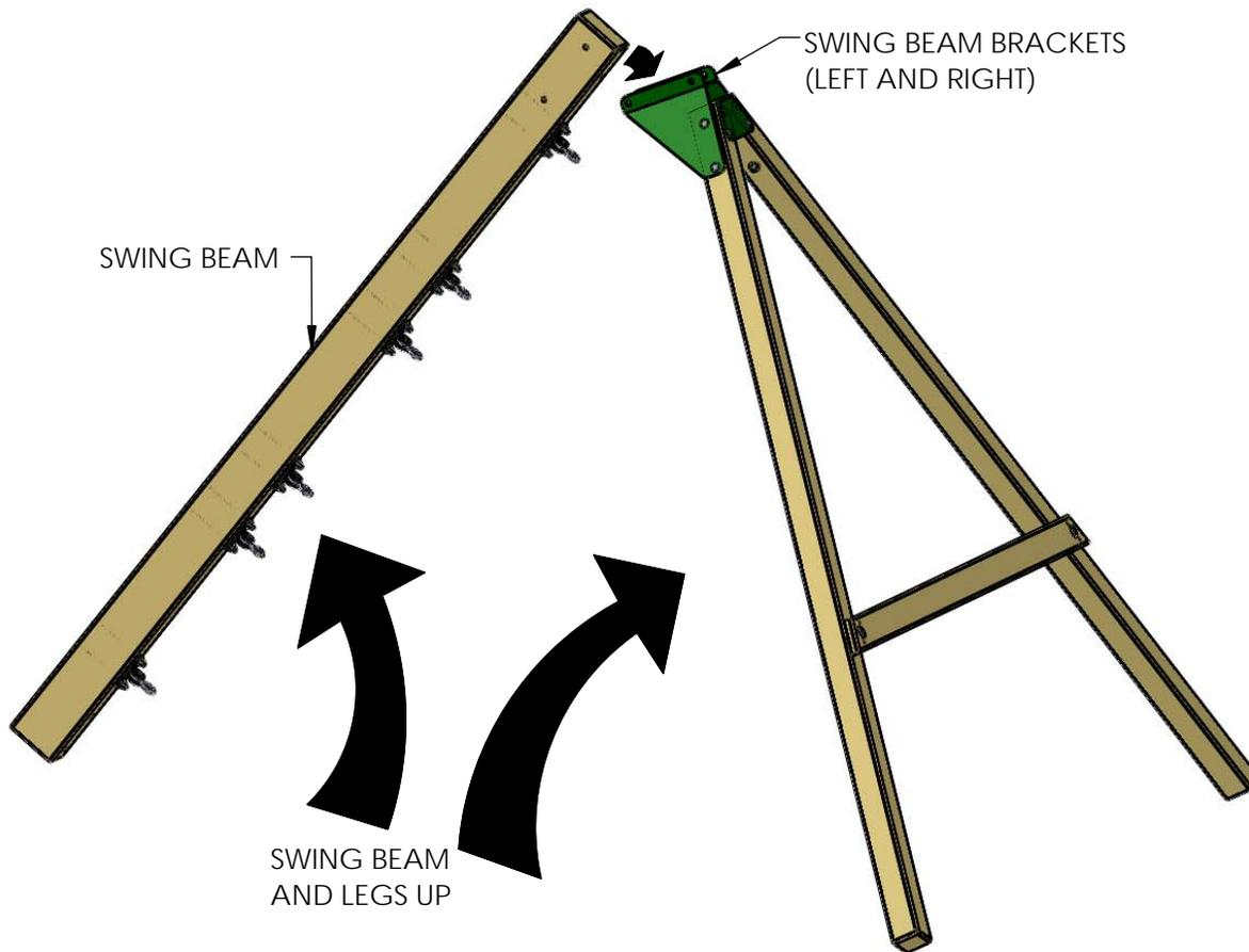
2: ASSEMBLE WITH FASTENERS AS SHOWN
