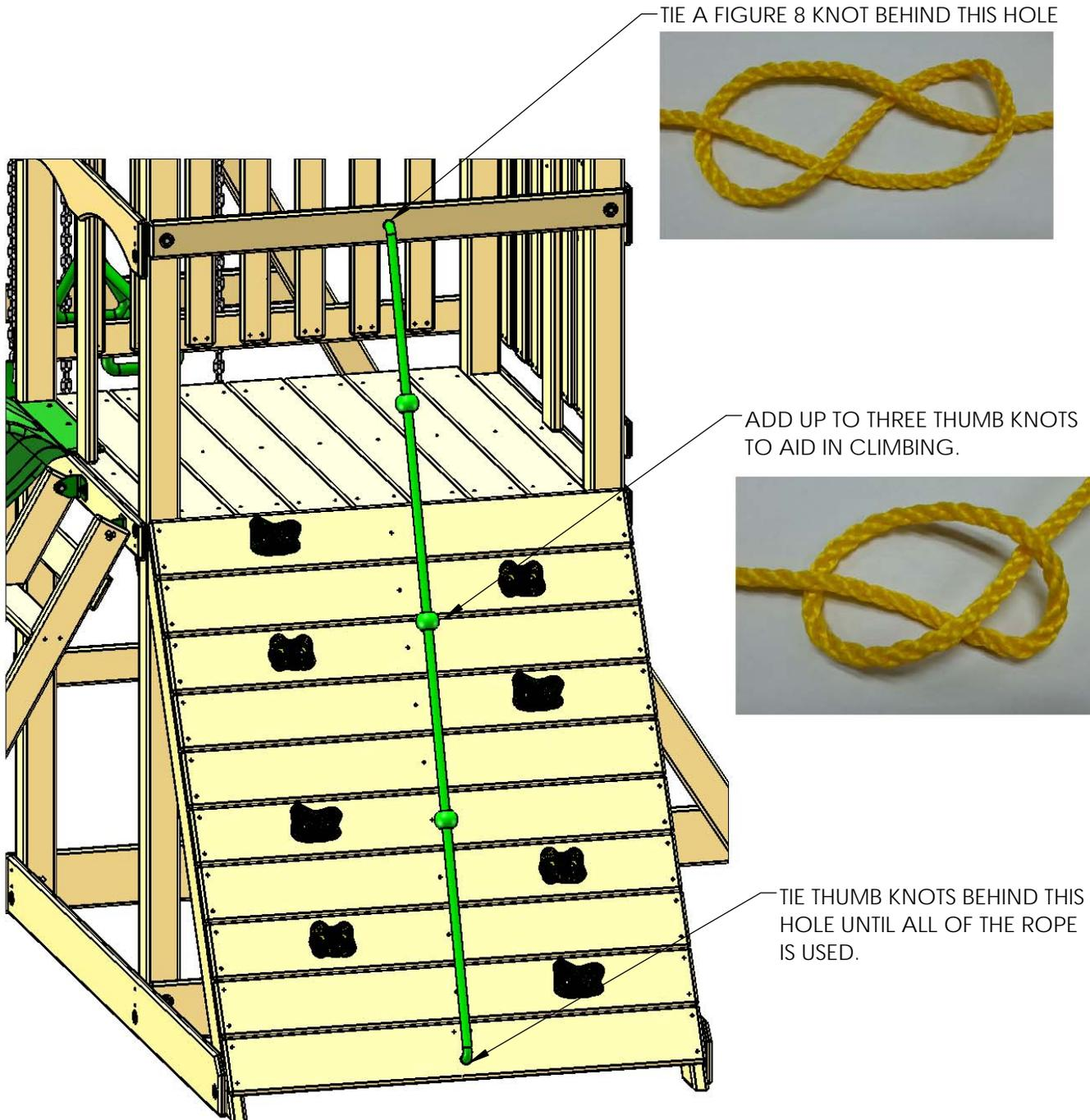
**FOR SAFETY, ENSURE THAT THE ROPE IS TIGHT ENOUGH SO THAT IT CANNOT BE LOOPED BACK ON ITSELF.**
