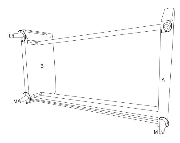
3. SCREW IN THE LEGS TO ASSEMBLE ONTO THE ARMRESTS. PAY ATTENTION TO FRONT AND BACK LEGS ARE DIFFERENT.
