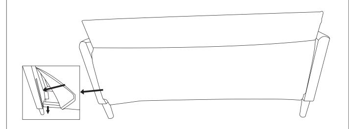
9.ATTACH THE BACKREST COVER(J) TO UNDER-SEAT CONNECTION BAR(N) AND ARMRESTS(A&B) BY USING THE VELCRO. MAKE SURE IT IS STRAIGHT AND SMOOTH.
