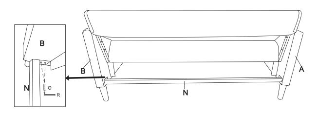
8. SCREW IN THE BOLTS(OX4PCS) TO ASSEMBLE UNDER-SEAT CONNECTION BAR(N) AND ARMRESTS(A&B). DO NOT TIGHTEN ALL BOLTS TO 100% UNTIL ALL BOLTS ARE IN CORRECT POSITIONS.
