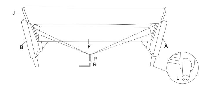
7. SCREW IN THE BOLTS(PX4PCS) TO ASSEMBLE THE BACKREST FRAME(F) AND ARMRESTS(A&B). DO NOT TIGHTEN ALL BOLTS TO 100% UNTIL ALL BOLTS ARE IN CORRECT POSITIONS.
