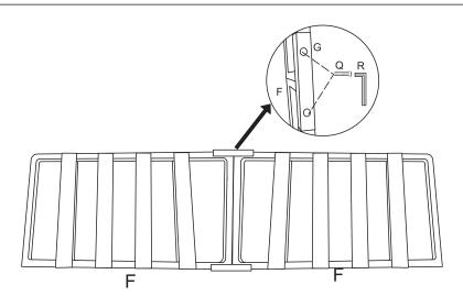
5. SCREW IN THE BOLTS(QX4PCS) TO ASSEMBLE THE BACKREST FRAME(F) AND THE CONNECTION BAR(G). MAKE SURE ALL BOLTS ARE TIGHTEN TO 100%.
