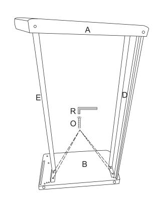
2. SCREW IN THE BOLTS(OX4PCS) TO ASSEMBLE ARMREST LEFT-HAND SIDE(B) / SEAT FRONT PANEL(D) AND SEAT BACK CONNECTION BAR(E). TIGHTEN ALL BOLTS TO 100%.
