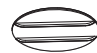
DD Cap x1 Use when cleaning & painting or when fixture is not in use
