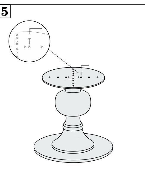
At First, Place the connecting plate on the base.
