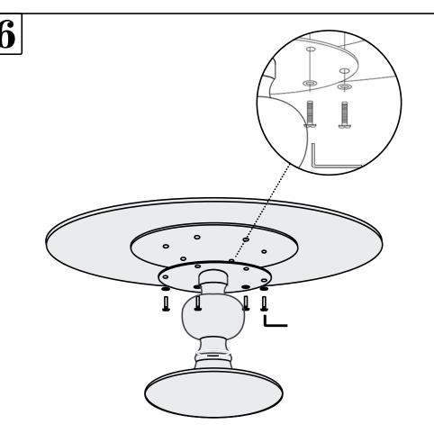
After the holes in the three parts of the desktop, connecting plate and chassis are aligned, we can start to tighten the screws against the holes.
