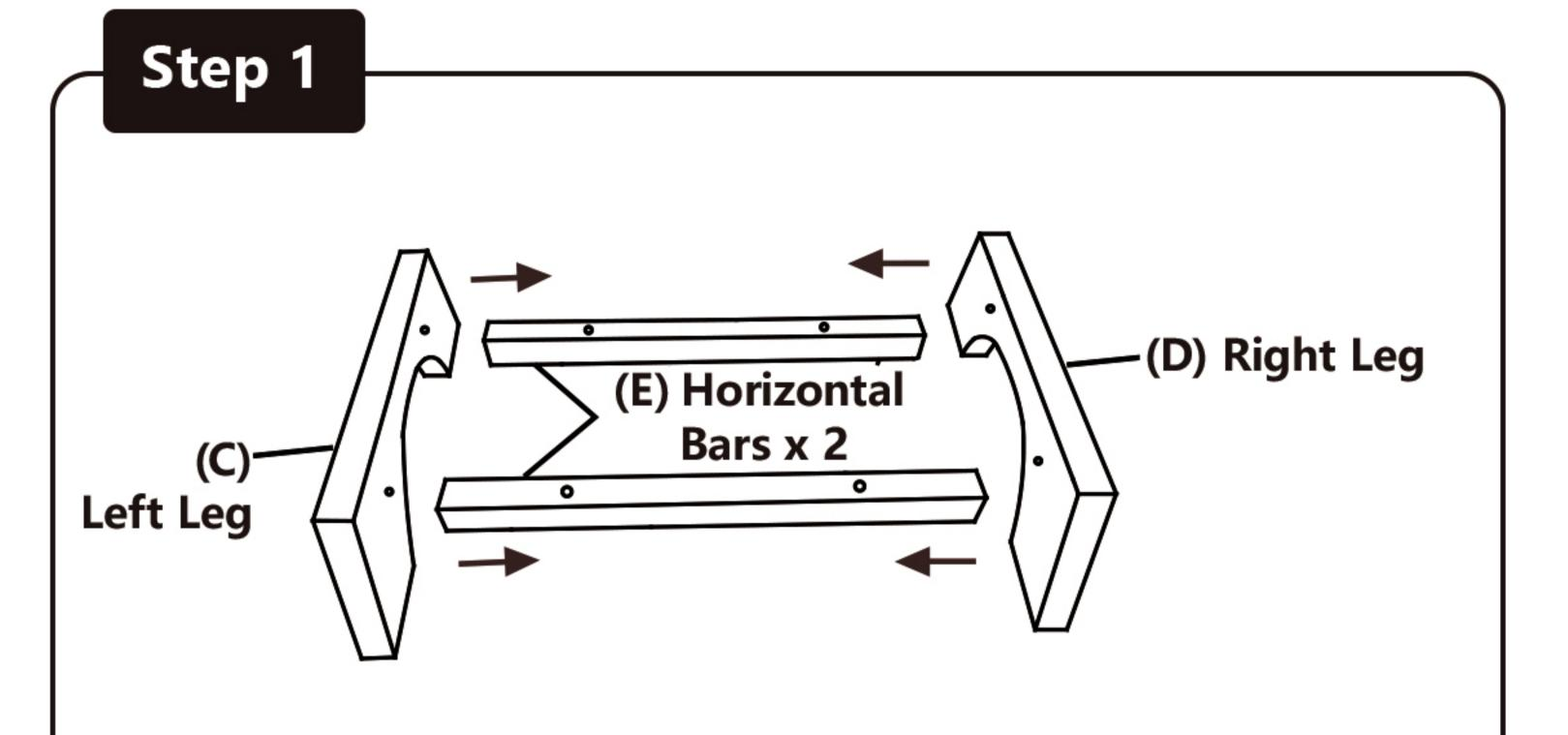
Place the Left Leg (C) and Right Leg (D) symmetrically, and align them with the four holes on the sides of 2 Horizontal Bars (E)
