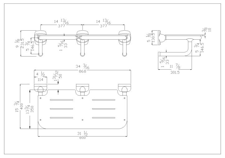
Rectangular shower seat manufactured with heavy duty coated frame and phenolic platform
