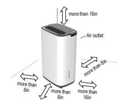
• Allow at least 8 inches of air space on all sides of the unit for air circulation (at least 16 inches for air outlet).
