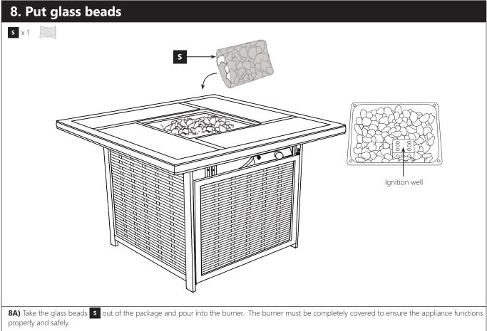
**Warning:** The ignition well MUST be clear and fire of obstrucions at all times to insure proper operation. DO NOT cover the ignition well with any glass beads or other media.
