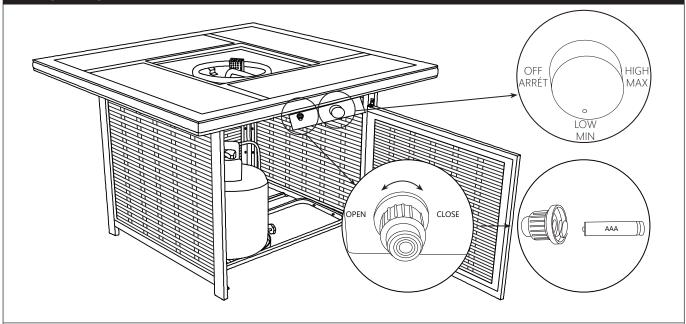
**2A)** Turn on the gas supply, ignite the burner, and test at all connections for leaks using a soapy water solution. If bubbles appear, a leak is present. Turn off the gas and tighten at all connections. Repeat until no leaks are present. If a leak persists, turn off the gas supply and contact the local gas company or dealer.
