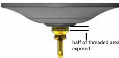
Drawing 2 – Canopy Adjustment
