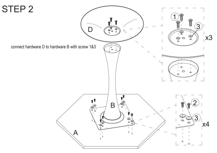
connect hardware A to hardware C&B with screw 2&3
