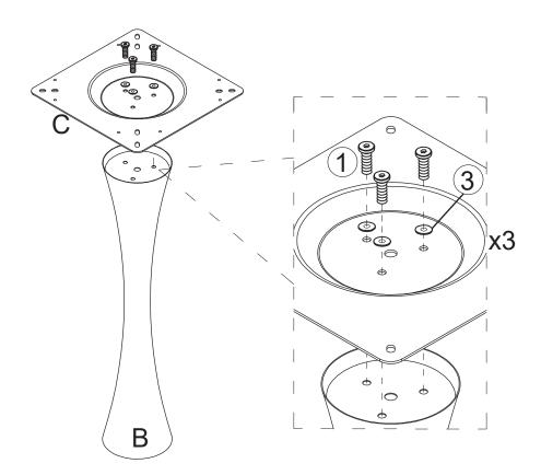
connect hardware C to hardware B with screw 1&3
