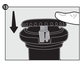
14. Align one of the cord clips with the power cord hanging over the rim of the bowl. With the two-prong end on the outside of the bowl, slide the cord clip down until it clips onto the bottom of the bowl.
