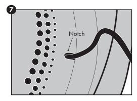
Remove the flow control cap from the filter housing by gently lifting up. Do not twist to remove it.
