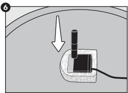
Align the cone so the cord runs through the notch without moving the pump from its original position. Once the cord is aligned, gently place the cone piece into resting position.
