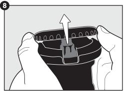
Rinse the carbon filter thoroughly under cold water to remove any loose carbon dust. Unscrew the filter housing cap and insert the carbon filter into the filter housing with the pull-tab facing up. Then, screw on the filter housing cap.
