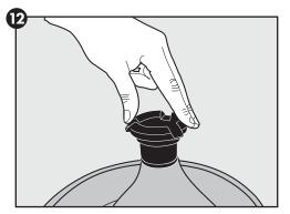
13. Align the flow control cap with the raised notches on the filter housing cap and press down to secure in place. Turn the flow control cap to the right to increase the flow of water and turn it to the left to decrease the flow.
