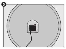
6. Place the intake tube into the circular opening on the top of the pump.
