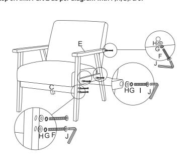
Step 6: Tighten all screws then assembly is complete.
