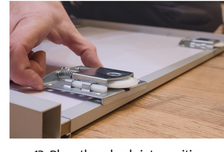
12. Place the wheels into position at the bottom of the frame
