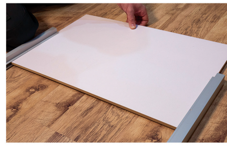
9. Slide all the remaining wooden panels and mid rails into position within the door frame
