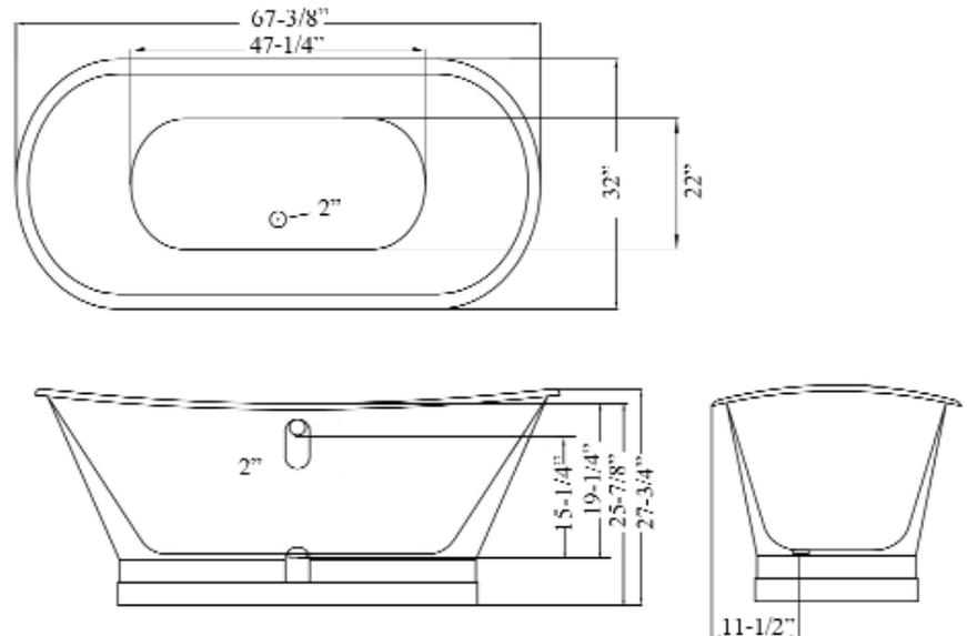
Dimensions of fixture are nominal and may vary within the range of tolerances established by ANSI Standard A112.19.2. Dimensions and specifications subject to change without notice.
