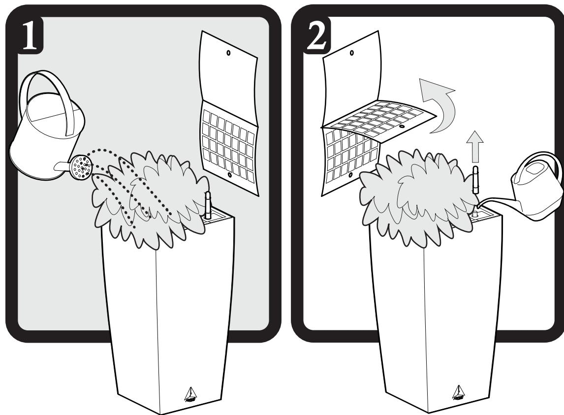
To establish root development, water from the top for the first month. Once roots have grown to the bottom of the plant water tray, fill through the water tube.
