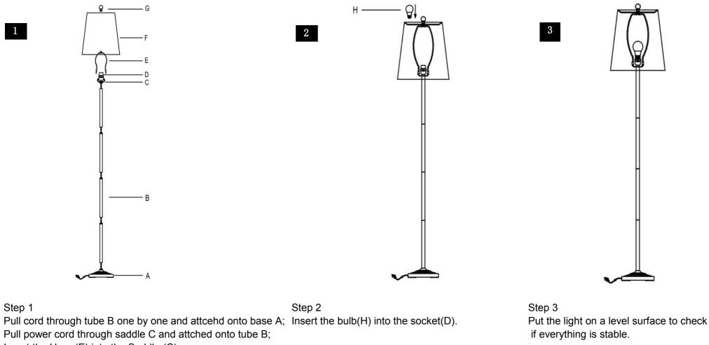
Insert the Harp (E) into the Saddle (C).
