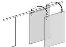
(B) Next, Put pulley B on the track, so that the pulley B and pulley A cross. As shown in the figure below.
