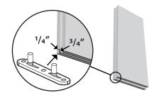
Install the hangers onto the door according to the measurement in the pictures below. Before doing this, remove the anti-bouncer from the pulley. Maximum door thickness is  $2^{3}/_{8}$ ". If your door's thickness is less than 2", please use the short door bolts(2"). If your door's thickness is more than 2"and less than  $2^{3}/_{8}$ ", use the long door bolts ( $2^{3}/_{8}$ ").
