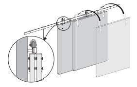
As shown in the figure, after all the pulley blocks are connected to the track, the anti-bouncer are fixed with hexagonal screw rod.
