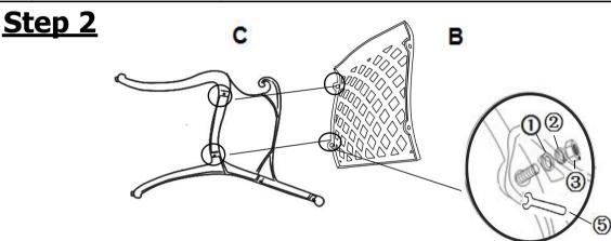
Attach the Chair Seat Panel(B) to the Left Leg with Arm (with preattached Levellers) (C) using Washers(1), Spring Washers(2) and Nuts(3), with Spanner(5).
