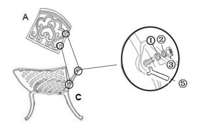
Then attach the Backrest Panel(A) to the top end of the Left Leg with Arm (with pre-attached Levellers) (C) using Washers(①), Spring Washers(②) and Nuts(③), with Spanner(⑤).
