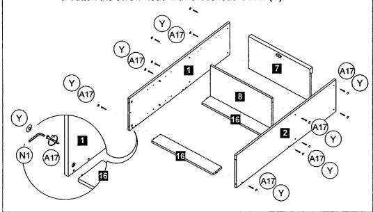
STEP 10 Use Allen Key (N1) to tighten the Crosshead Screw 6.3 x 40mm (A17) & button the screw head with Crosshead Cover (Y).
