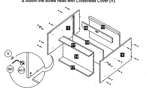
Assemble the upper unit to the main unit by using Mini Fix 15mm (F2) STEP 12 & cover the Mini Fix by using Mini Fix Cap (Y).
