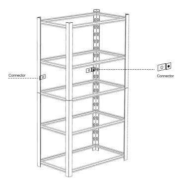
Use the connector to snap into the hole of the column, punch a hole on the wall, put the expansion screw in, and use the screw to pass through the connector to connect with the expansion screw
