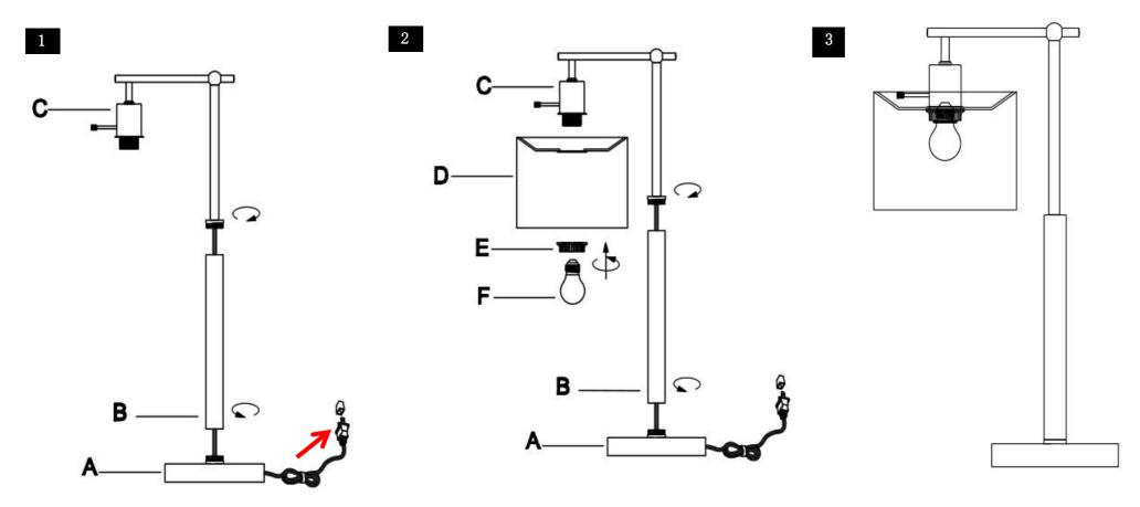
Step 1 Pull power cord to connect the Lamp body (B) to the Lamp basiPut the shade (D) on the Socket (C), then Screw the Lamp body (B) onto the Lamp base (A). Screw the Socket (C) onto the Lamp body (B). Be careful not to twist the power cord and tighten securely
