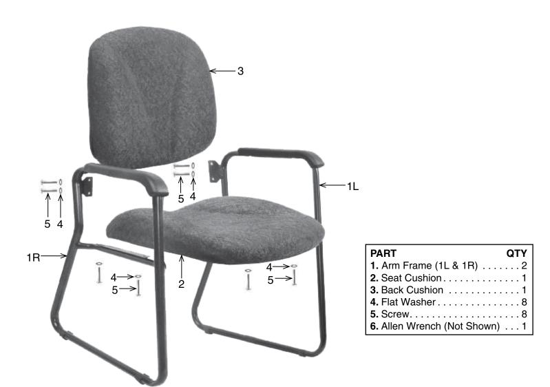
Remove all parts from carton, separate by part numbers indicated on parts list, and verify part quantities.
