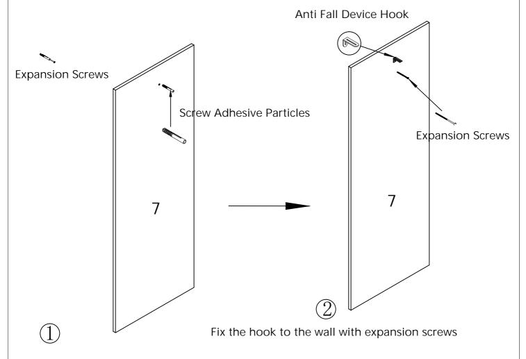
Drill a hole in the wall and then tap the expansion-screw adhesive into the wall
