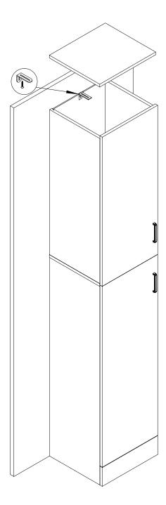
Install self tapping screws, connect hooks to small cabinet panels
