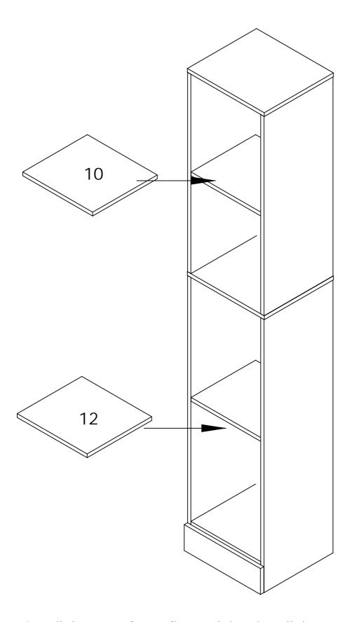
Install the outer frame first and then install the movable laminate
