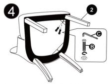
Put the screws in the holes, tight the screws, but not too tight, 90% is ok.
