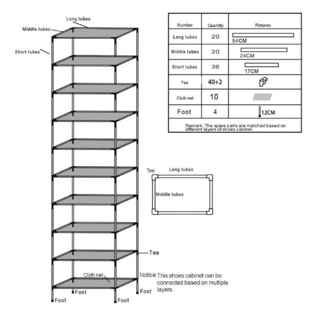
Taking out 4pcs plastic tee, 2pcs long rail tubes, 2pcs short rail tubes. Inserting plastic tee based on direction of arrows, then inserting small cloth to long rail tubes, lying flat, taking out 4pcs supporting tubes to insert plastic tee. According to pictures to connect:
