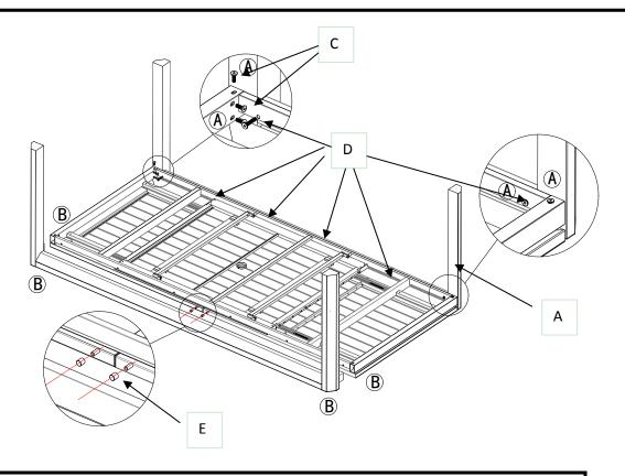
2. Properly tighten all the bolts (C) & (D). Carefully turn the table to the upright position.
