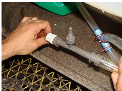
8. Insert the Ozone injector's large barbed ends into each end of the cut hose.
