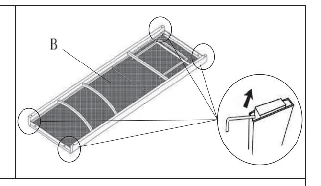
Open the carton and place all the parts onto a clean, non-marring surface. Remove the plastic plugs (prevent the alum tube was scratched) from the four ends of the Seat Panel(B) using Allen Key(③) as shown above. Place the Seat Panel(B) with its inside facing up.
