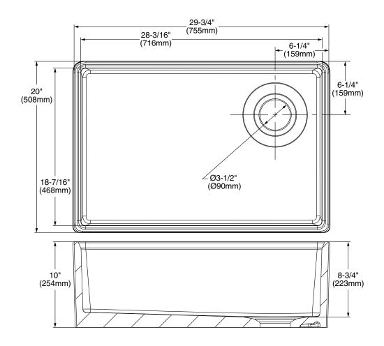
**NOTES:**\* DIMENSIONS SHOWN FOR LOCATION OF SUPPLIES AND "P" TRAP ARE SUGGESTED. FITTINGS NOT INCLUDED WITH FIXTURE AND MUST BE ORDERED SEPARATELY. SEALING COMPOUND SUPPLIED BY OTHERS.
