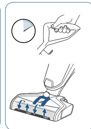
**5.** Each time you use the product, hold the solution trigger for 10 seconds to prime the system with cleaning solution before you begin cleaning. When you pull the trigger, LED lights will illuminate.
