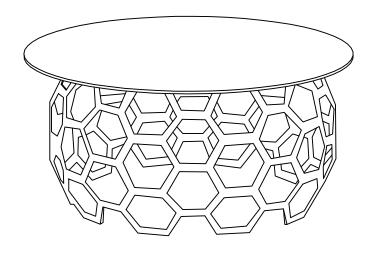
STEP:2. Place the Glass Top (B) onto the top of Iron base with Glass Sucker and make sure the top overhang is the same all around.
