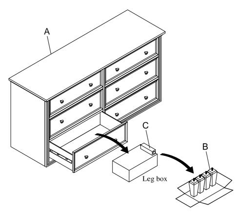
Turn upside down and place on soft surface. Attach Legs(B) & Center Support Leg(C) to Dresser(A).
