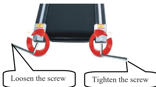
Picture B Adjustment Method for Right-sided Running Belt Deviation
