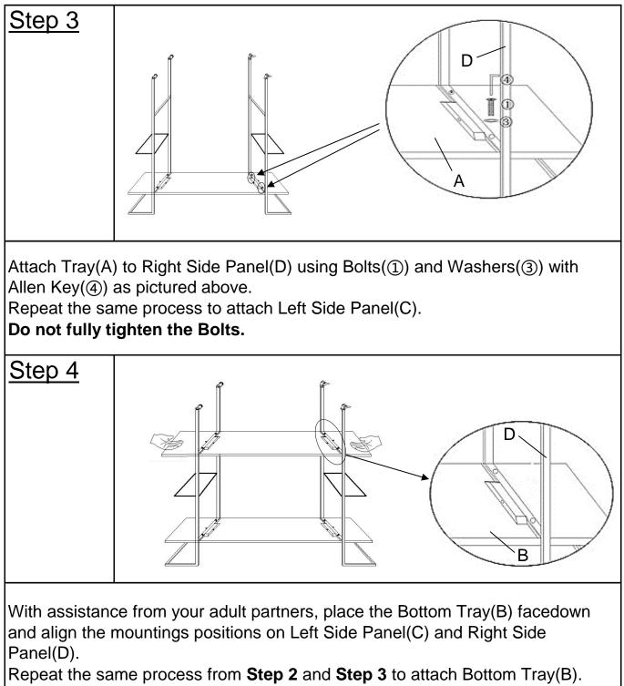
Now fully tighten all Bolts at all joints in a sequential manner.
