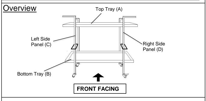
This Trolley has multiple parts and may require up to 30 minutes to assemble. To give you an overview of the Trolley parts, the above picture is to help you put the various parts into perspective. Please read through the instructions below to familiarise yourself with the parts and steps before assembly.
