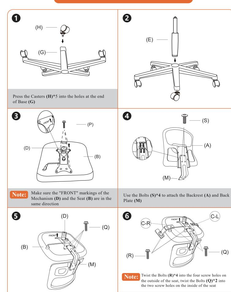
Use the Bolts (Q)\*4 to attach the Back Plate (M)
