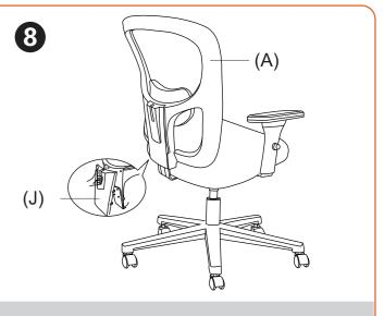
Buckle the Back Lid (J) into the slot of the Backrest (A)
