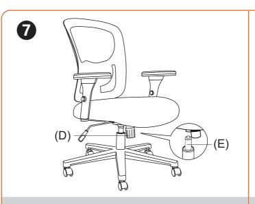
Align the hole on Mechanism (D) with Gas Lift (E), and press the Chair down until it is fully secured.
