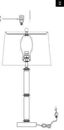
Step2 Insert the bulb(G) into the socket(C).
