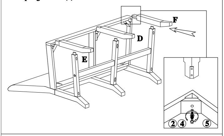
STEP 6: Fix stretcher (G,H,I) again by screw (7). Assembly complete
