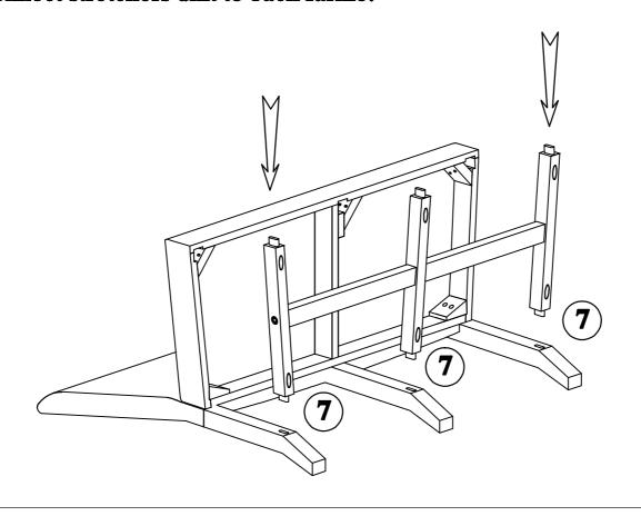
STEP 5: Insert 3 legs (D,E,F) to the unit. They are fixed by bolt (2) washer (4) and spring washer (5)
