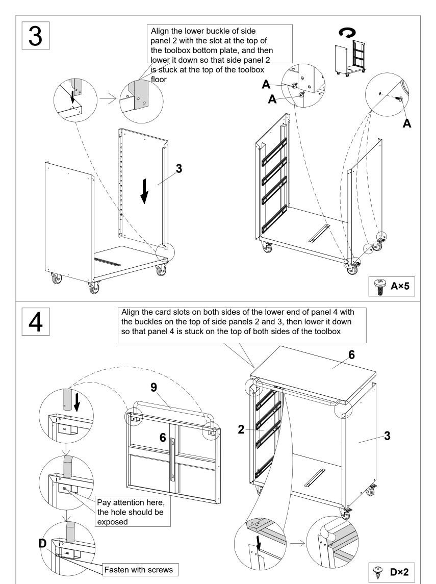
Fix component 4 with screws A according to the diagram
