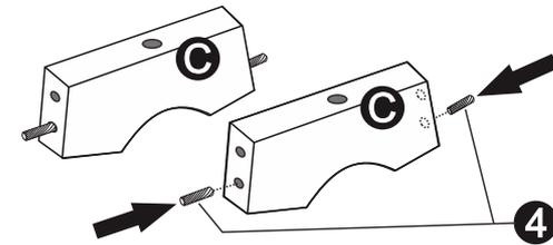
**STEP 1:** Insert wood dowel pins to end aprons.
