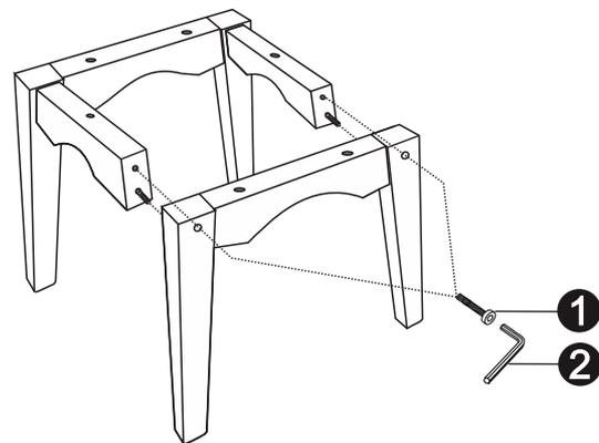
**STEP 3:** Connect end aprons to another side of legs by inserting wood dowel pins, then tighten screw (1) with allen key (2).
