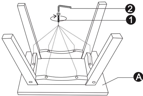
**STEP 4:** Assemble the lower part to table top with screw (1) and allen key(2).
