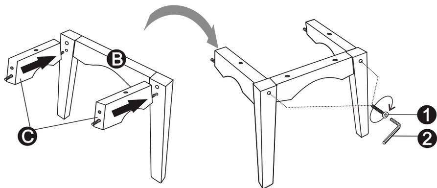
**STEP 2:** Connect end aprons to legs by inserting wood dowel pins, then tighten screw (1) with allen key (2).
