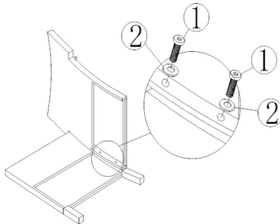
Open the carton and place all the parts onto a clean, non-marring surface. Attach the Backrest(C) to Left Armrest(A) using Bolts(①) and Washers(②) with Allen Key(③) as shown in the picture.
