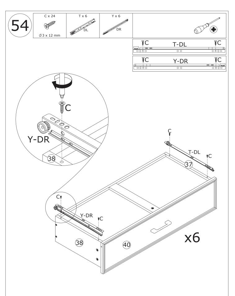
Assemble hardware T and Y to the drawer using hardware C as shown.
