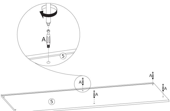
Attach hardware A to plate 5 as shown.
