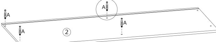
Attach hardware A to plate 2 as shown.
