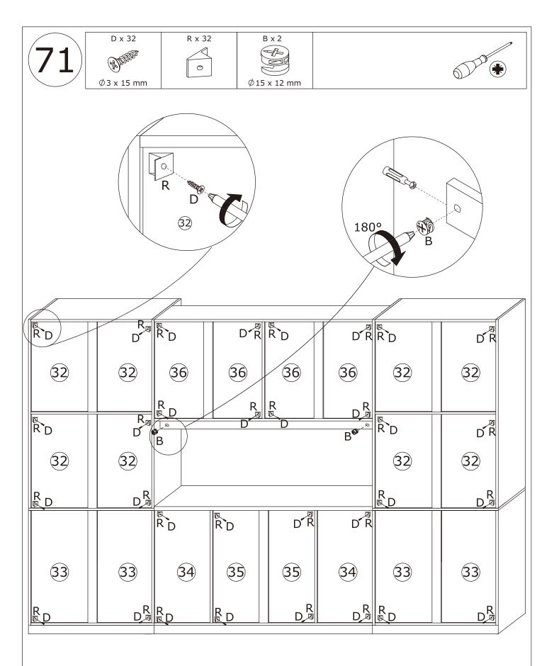
Secure the plastic part R to the top of theassembly with hardware D as shown.
