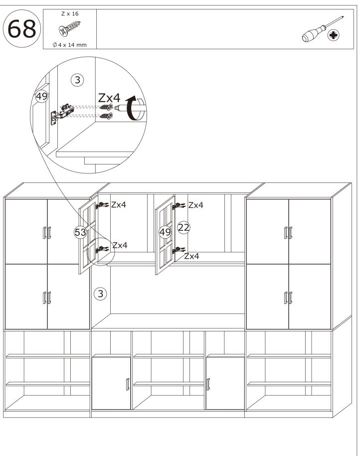
Assemble parts 49,53 to the assembly with hardware Z as shown.
