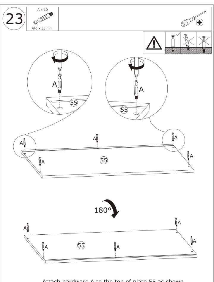
Attach hardware A to the top of plate 55 as shown.
