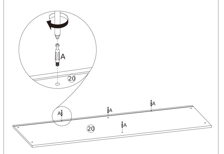
Attach hardware A to the top of plate 20 as shown.
