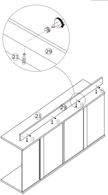
Secure part 29 to part 21 with hardware B as shown.
