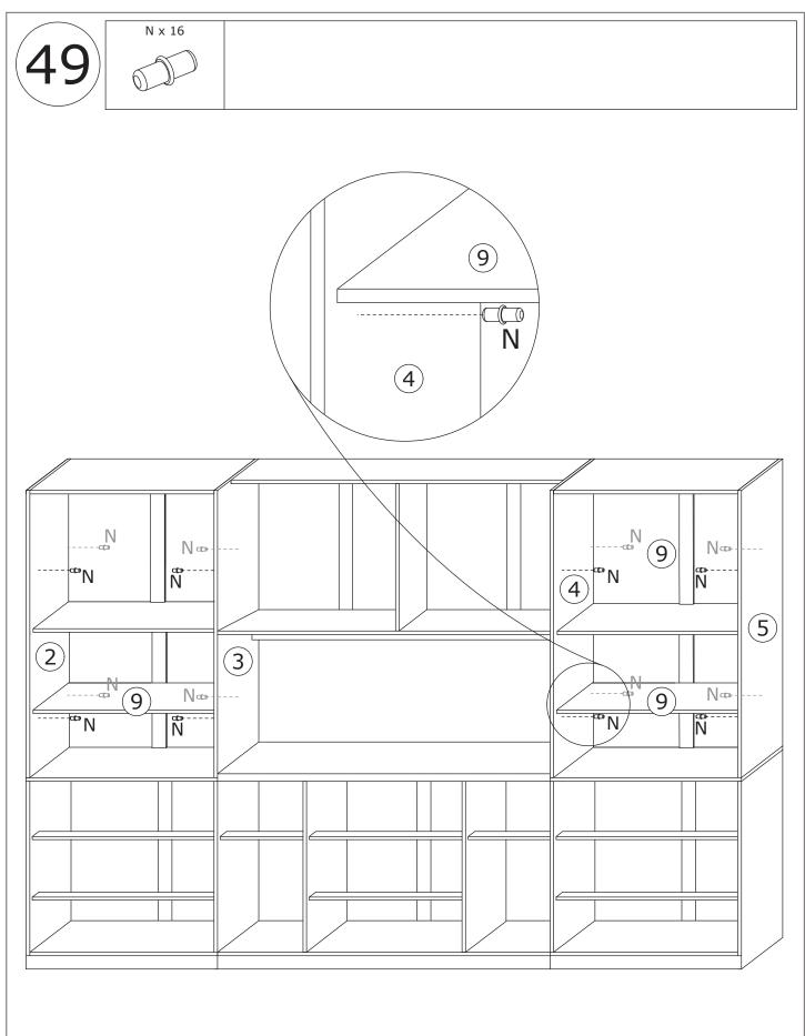
Assemble part 9 to the assembly with hardware N as shown.
