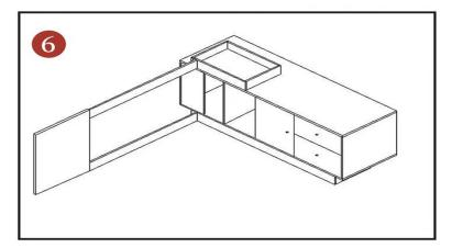
**STEP 6:** Front trim board link to side cabinet, trim board Need to install foot nails.
