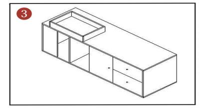
**STEP 3:** Cover the top plate and install the table support box.
