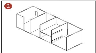
**STEP 2:** Install the bottom plate and neutral plate, neutral plate Pay attention to the order, the vertical plate of the guide rail is installed at the very edge.
