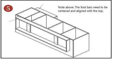
**STEP 5:** Attach the foot bar to the bottom plate with Self-tapping screw.
