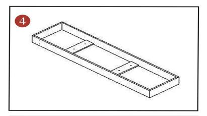
**STEP 4:** The foot strip at the bottom of the auxiliary cabinet, and install the foot nails.
