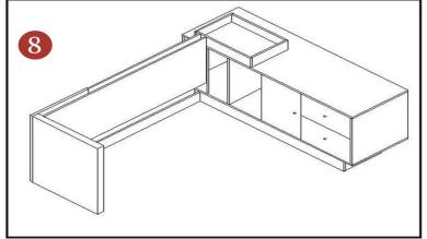
**STEP 8:** Start by linking the desk front to the foot lift Then link to the Side cabinet, The final decorative board is then linked to the foot lift, The bottom of the foot needs to be nailed.
