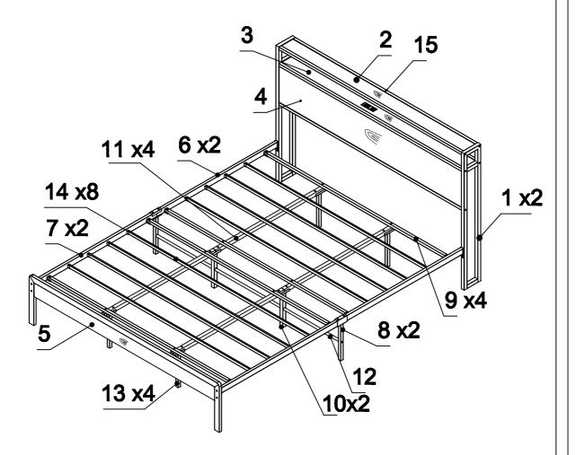
Please don't tighten the screws completely and go back later for a final tightening of all the screws after pieces are aligned with each other.
