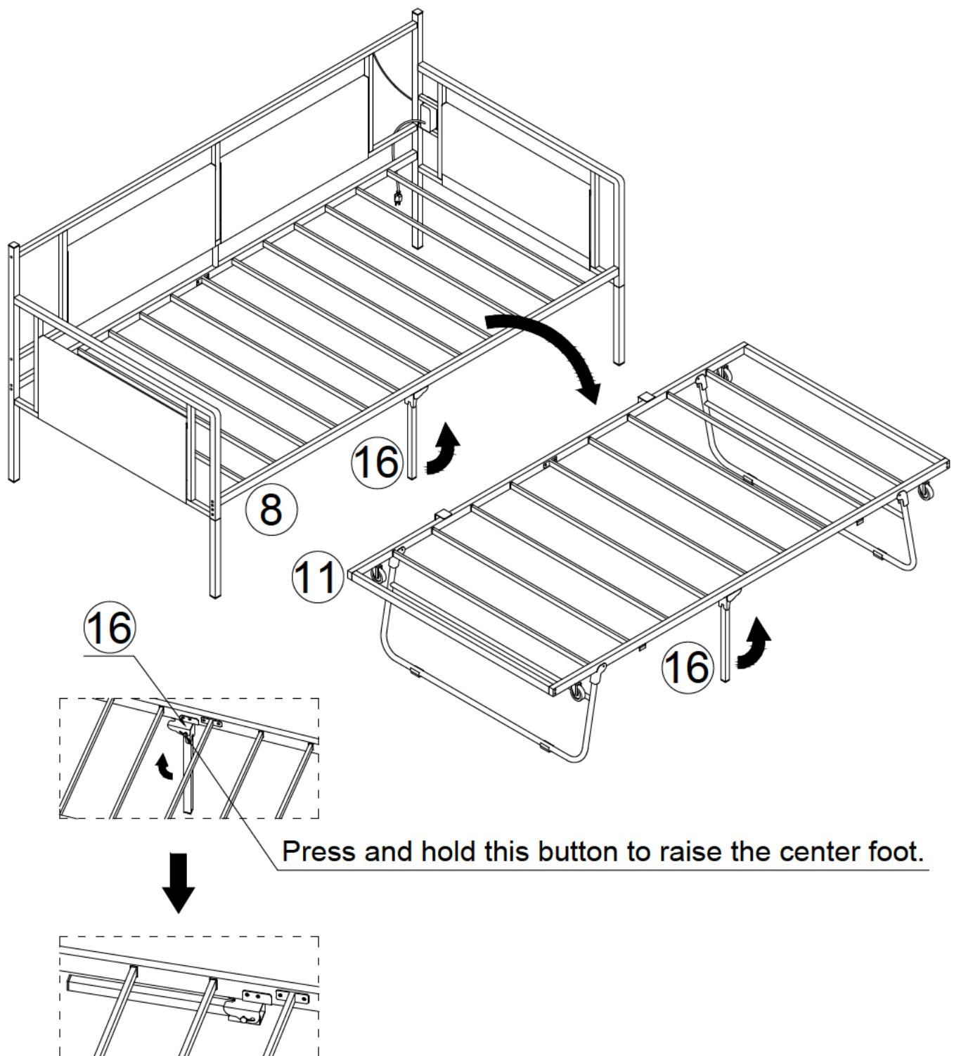
Note: Take the #11 tube out of the #8 tube and rotate the #16 center leg up.
