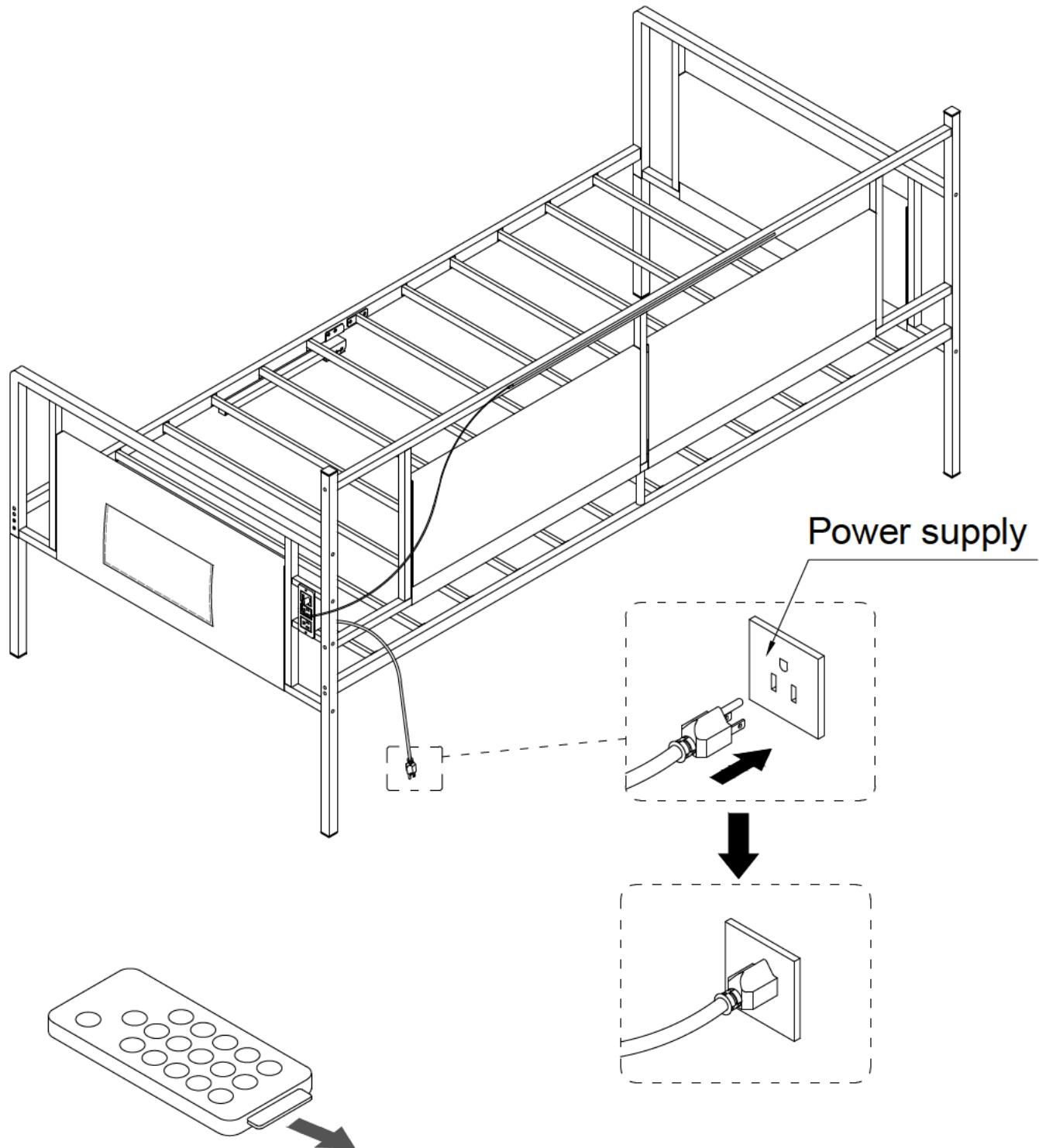
Note: The remote control can be used by pulling the plastic piece at the bottom of the remote control outward.
