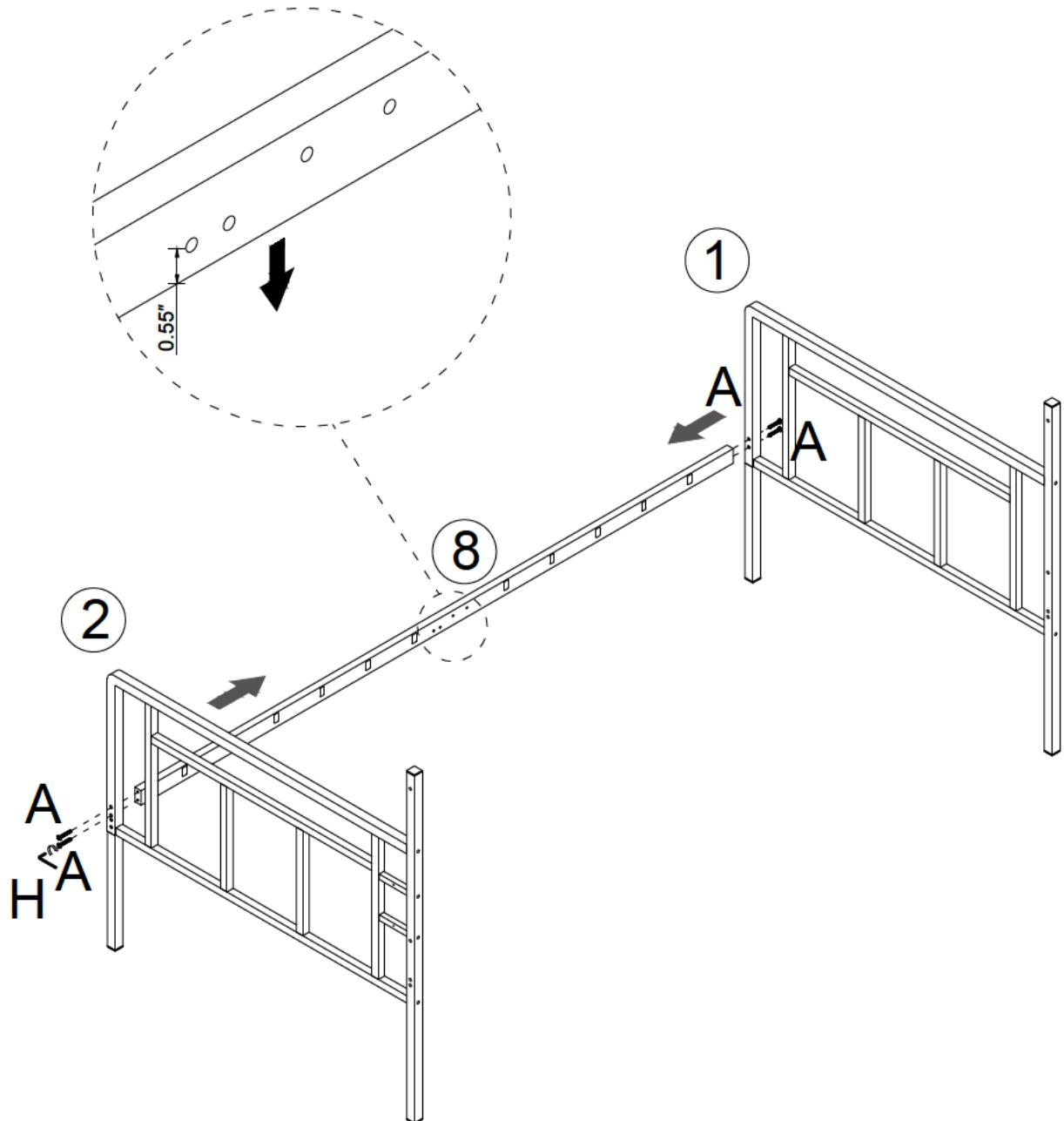
Note: Hole spacing is 0.55 inches down as shown.
