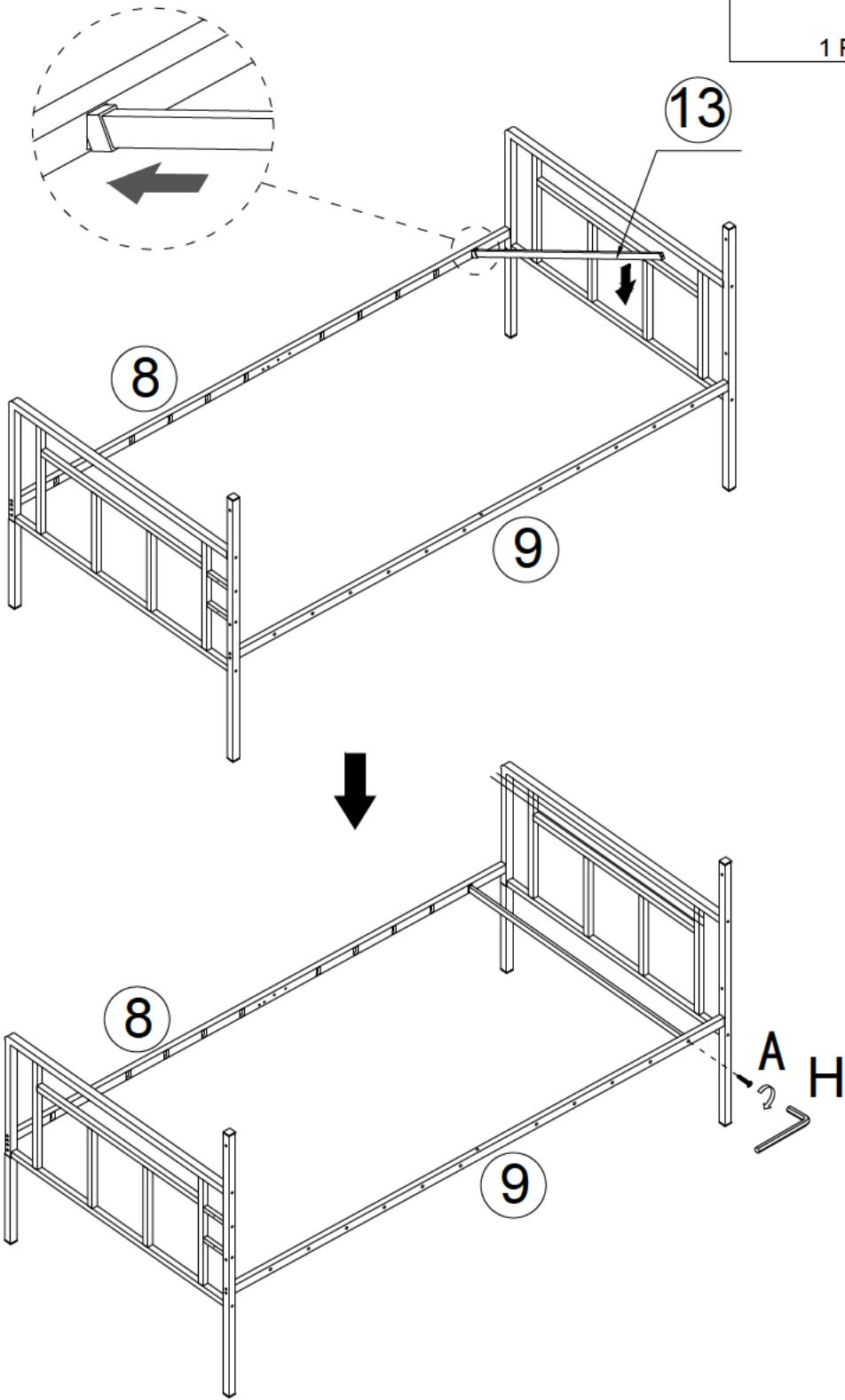
Note: Screw A is tightened to 80%.
