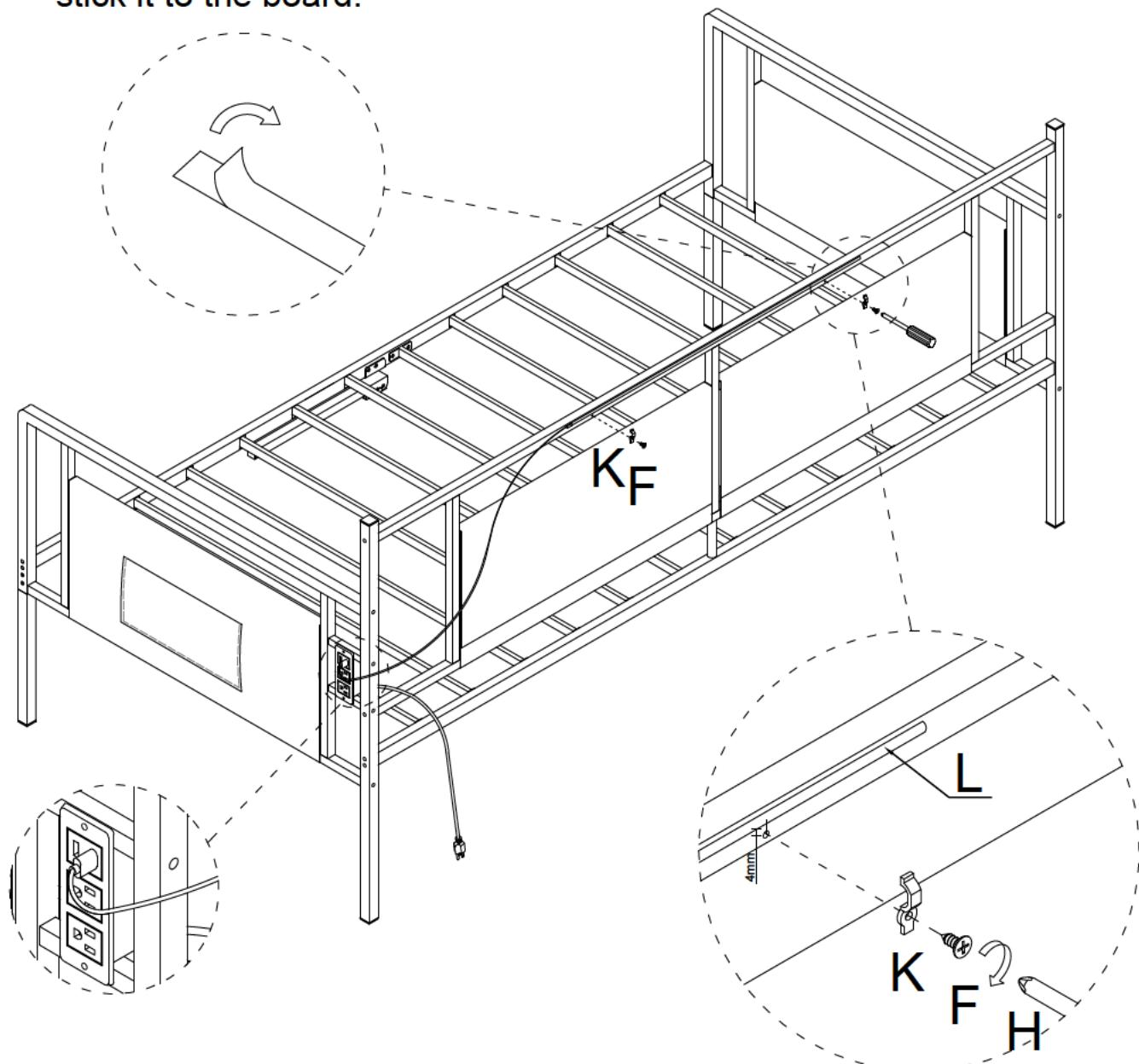
Note: When pasting, leave a gap of about 4mm with the center of the hole to paste.
