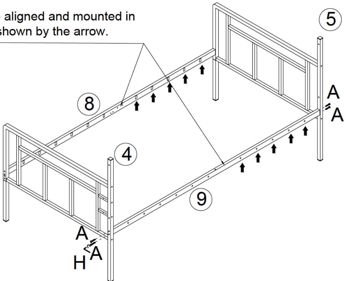
Note: Screw A is tightened to 80%.
