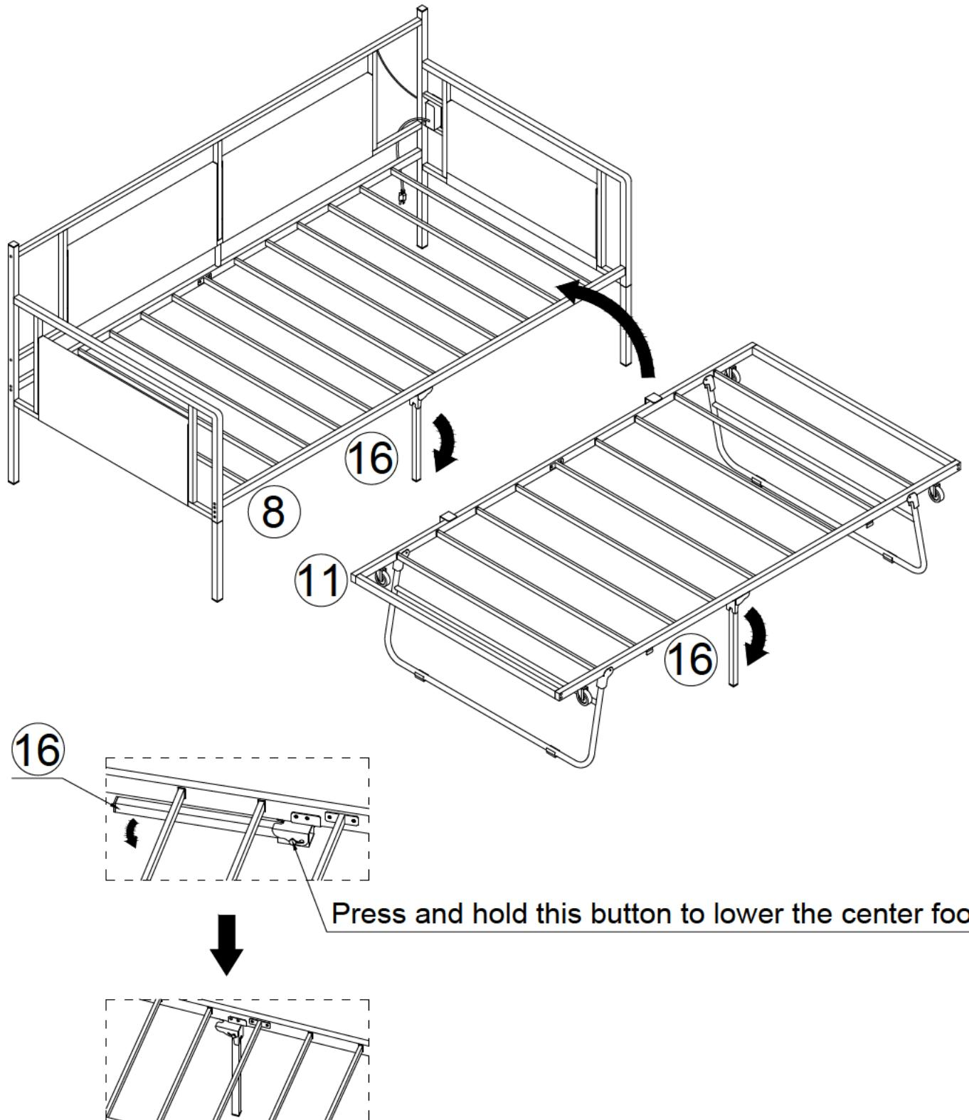
Note: With the 16 gauge center down, hook the 11 gauge tube to the 8 gauge tube.
