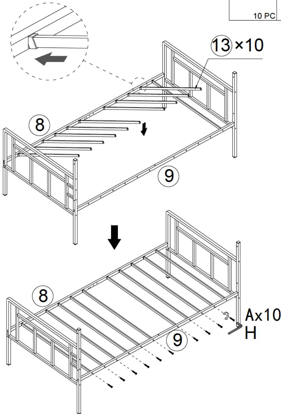
Note: Screw A is tightened to 80%.
