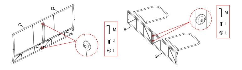
2. Secure chair arms (A&B) to assembled chair back (C&D) with 4 washers (L) and 4 screws (I) by using allen wrench (M). Do not tighten all screws now.
