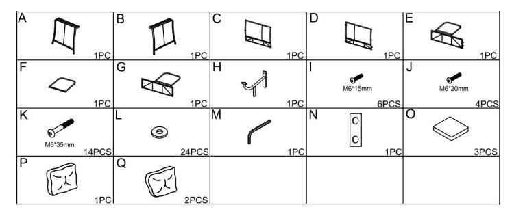
1. Attach two chair backs (C&D) to each other and two front panels (E&G) to each other with 4 washers (L), 4 screws (J&I) by using allen wrench (M). Do not tighten all screws now.
