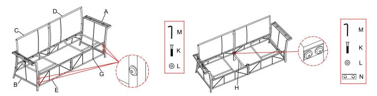
4. Secure seat panel (F) to support bar (H) and assembled front panels (E&G) and with 4 washers (L) and 4 screws (J&K) by using allen wrench (M). Do not tighten all screws now.
