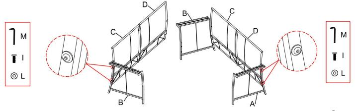
3. Secure assembled front panels (E&G) to chair arms (A&B) and support bar (F) to chair back (C&D) with 7 washers (L&N) and 6 screws (K) by using allen wrench (M). Do not tighten all screws now.
