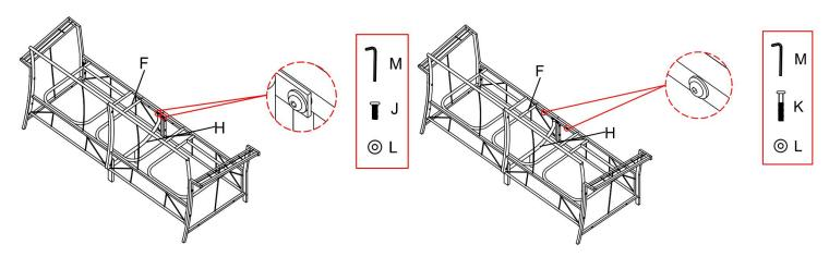
5. Secure assembled seat panel (E, F&G) with 6 washers (L) and 6 screws (K) by using allen wrench (M). Fully tighen all screws now and put cushion (O, P&Q) onto sofa.
