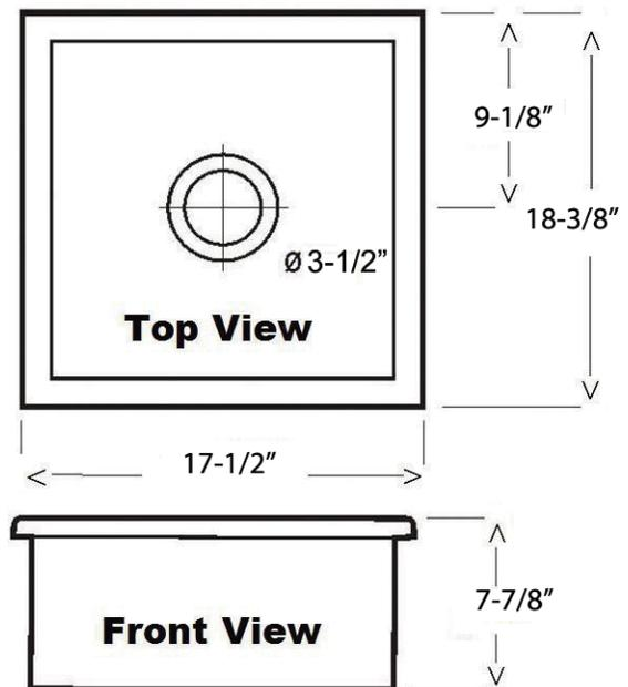
Dimensions of fixture are nominal and may vary within the range of tolerances established by ANSI Standard A112.19.9. Dimensions and specifications subject to change without notice.
