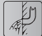
Flush the pipe
